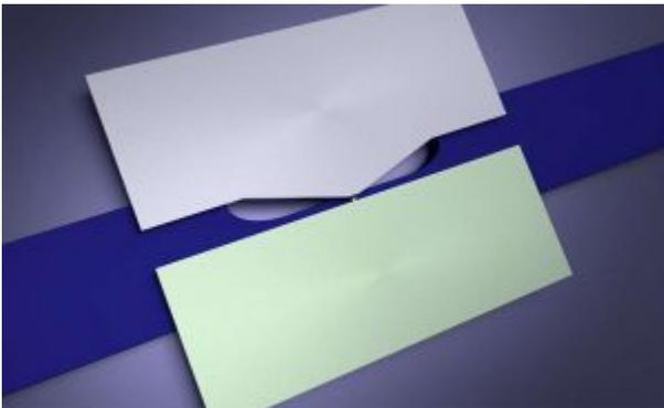
[Tiny plates made of silver \(light grey\) and platinum \(mint\) are placed on an optical waveguide \(blue\)](#)
