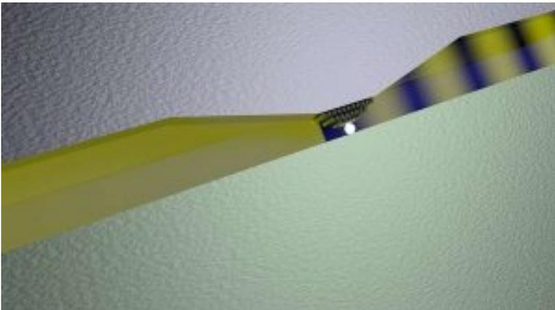
The switch is based on the voltage-induced displacement of one or more silver atoms in the narrow gap between a silver and a platinum plate.
