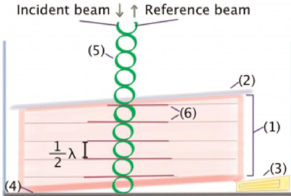
Holographic fabrication. A photosensitive emulsion (1) coated on a glass slide (2) is placed inside a tray with a 7° spacer (3) and facing towards a reflecting mirror (4). Upon exposure to the laser irradiation (5), the gold nanoparticle grains are arranged in fringes (6) align in parallel to the surface of the polymer, and are separated by half the distance of the wavelength they were exposed to. The diagram is not to scale.
