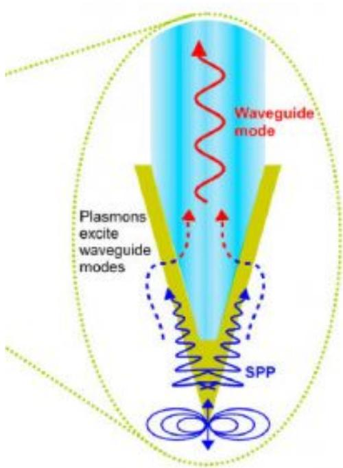
Tugchin et al., study experimentally the excitation of the radially polarized conical surface plasmon polariton (SPP) in a fully metal-coated conically tapered M-profile fiber which works as a “plasmonic tip” for the scanning near-field optical microscope (SNOM). This structure extends the Kretschmann configuration to the conical geometry. In this plasmonic tip, the radially polarized waveguide mode, propagating inside the
