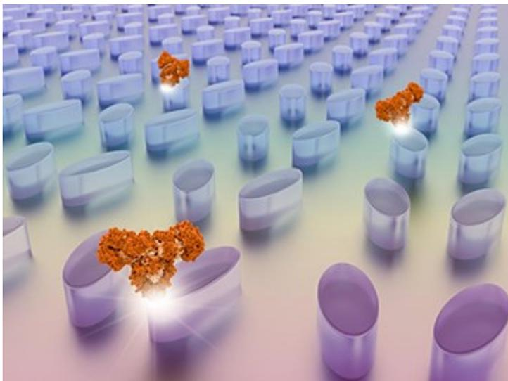
The detection platform demonstrated by scientists in Switzerland and Australia, which combines a high- $Q$ -factor dielectric surface and hyperspectral imaging, can reportedly detect biomolecules at a density of less than three molecules per square micron of detector.
