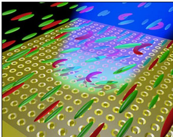
Schematic of the tunable color filter. The combination of a gold film with ring-shaped holes and the use of liquid crystals (red and green) enables pixels of a defined color that can be turned on and off. ©2012 Y.J. Liu
