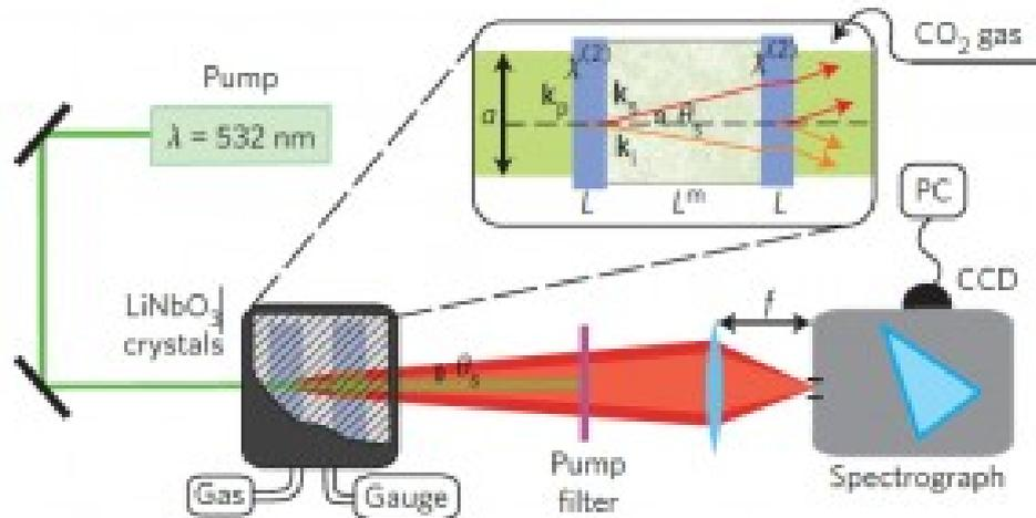
Experimental set-up. A continuous-wave laser at 532 nm pumps two nonlinear crystals, where SPDC occurs. The crystals are placed in a vacuum chamber and  $\text{CO}_2$  is injected into the chamber. The interference pattern of the SPDC from the two crystals is imaged by a lens onto a slit of a spectrograph and recorded by a charge-coupled device (CCD) camera.
