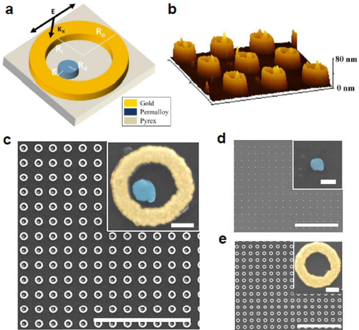
Magnetoplasmonic NCRD ferromagnetic-nanoantenna/gold-nanocavity and parent Py-DI and Au-RI nanostructures. a Schematic of the NCRD hybrid structure with its four geometric characteristic parameters. b Atomic force and c SEM images of the individual NCRD nanocavity and array. SEM images of the parent single d Py-DI, e Au-RI constituents and arrays. The scale bars in panels c-e correspond to 5  $\mu\text{m}$  and those in their insets to 100 nm.
