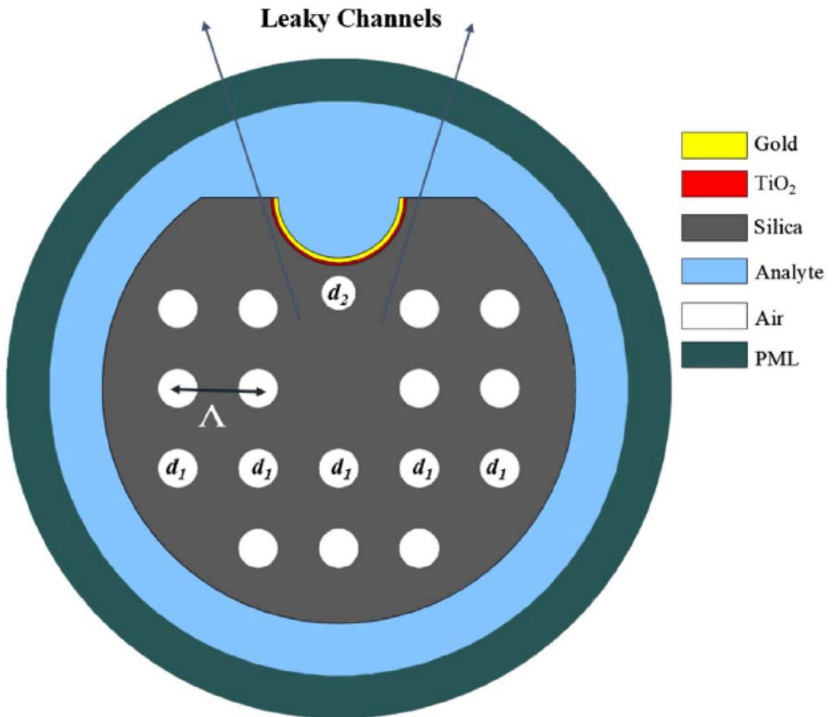
**Fig. 1.** Schematic diagram of the proposed sensor.
