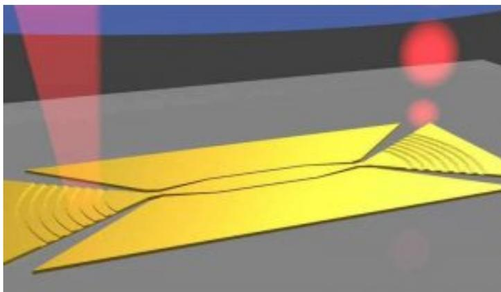
[Schematic representation of the metallic modulator: Left: a continuous beam of light strikes a metallic lattice that deflects the light onto the chip. Right: an optical data pulse exits the component.](#)
