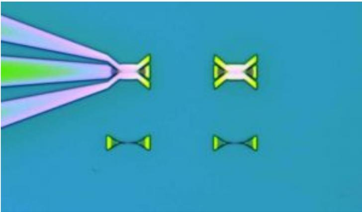
Microscopic image of a chip. Top left: functional modulator with electrical contacts; right: test modulator without electrical contact; below: test components.
