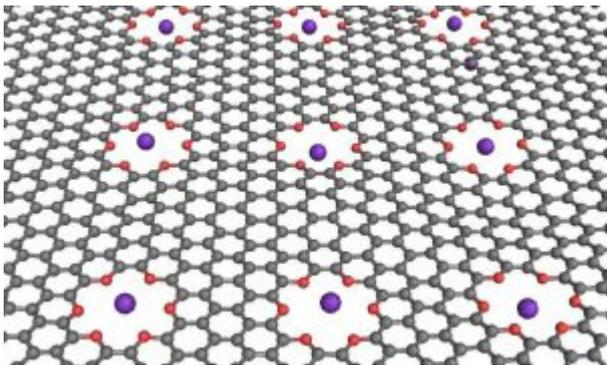
Invigorating the idea of computers based on fluids instead of silicon, researchers at the National Institute of Standards and Technology (NIST) have shown how computational logic operations could be performed in a liquid medium by simulating the trapping of ions (charged atoms) in graphene (a sheet of carbon atoms) floating in saline solution. The scheme might also be used in applications such as water filtration, energy storage or sensor technology.
