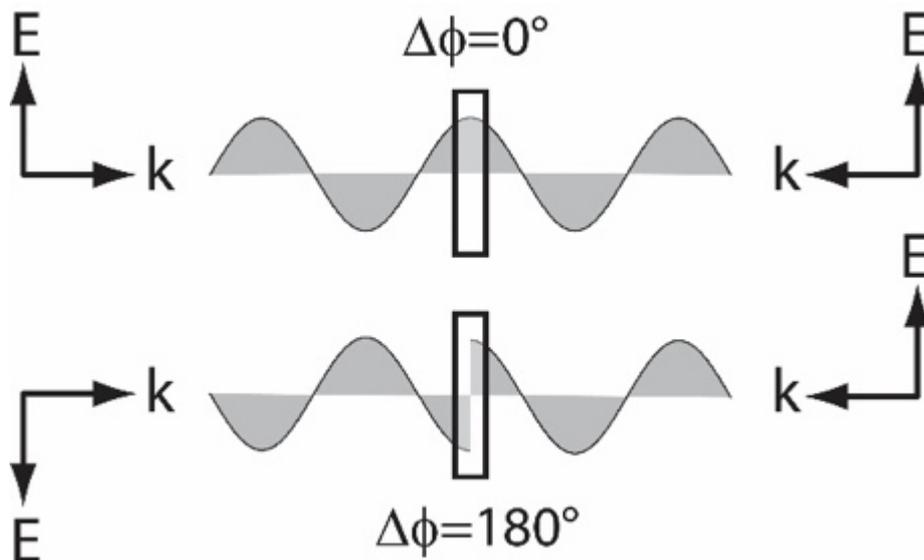
*Traditional “reverse lasers” can only absorb energy when the incoming electromagnetic waves are perfectly aligned, as in the top example. Courtesy of Kebin Fan and Willie Padilla, Duke University.*
