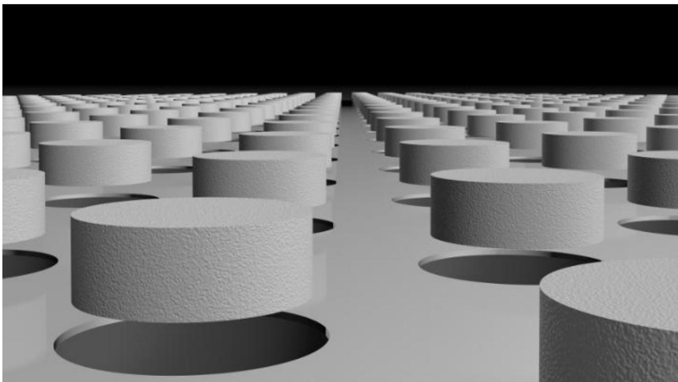
*The width, height, and spacing of the cylinders depicted here dictate how the metamaterial described in the new paper absorbs electromagnetic energy. Courtesy of Kebin Fan, Duke University.*
